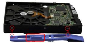
1. Each Hard drive requires using 2x HDD rail on each side.
